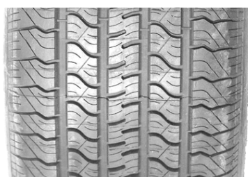
Figure 19. Tread pattern of the SRTT tyre
