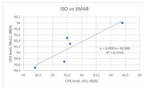
Figure 7b. Linear regression between ISO and SMA8
