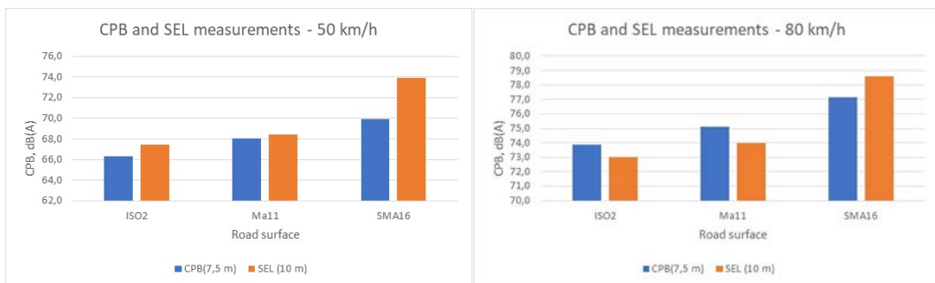
Figure 17. Measured noise levels from CPB and SEL at 50 km/h (left) and at 80 km/h (right) on 3 road surfaces. Average of 5 tyres.
